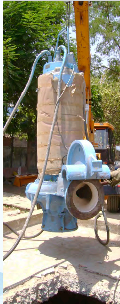
Air Cooled Motor - Conventional Pumpsets require Costly & Spacious Pump Rooms
